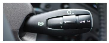
The shift lever includes gear, auto/manual mode and engine brake selection for excellent ergonomics.
